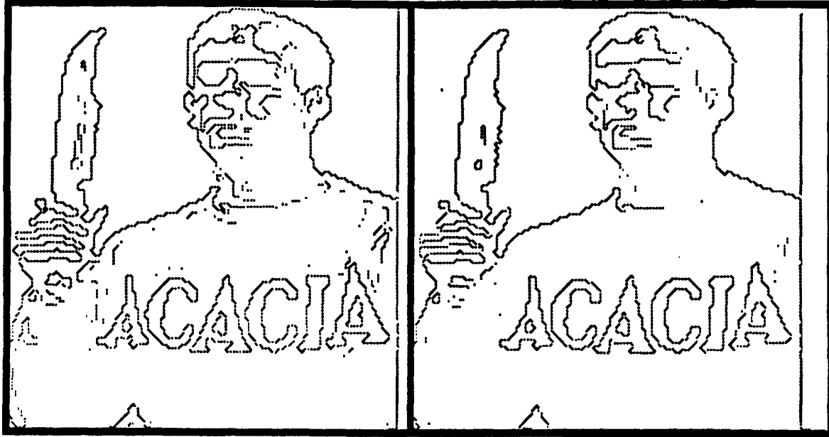
Figure 7: Zero-crossings from the difference of two Gaussians (left) and similar output from a difference of decaying exponentials (right).
