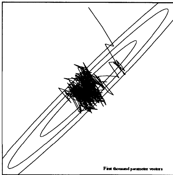
Figure 4: Delta-bar-delta (Jacobs, 1988) was apparently developed for use with deterministic gradient descent. It is also useful for stochastic problems with little noise, which is however not the case for this test problem. In this example \eta increases from its initial value, and then stabilizes. We use the algorithm exactly as it appears in Jacobs' paper with noisy gradients substituted for the true gradient (which is unavailable in the stochastic setting). Parameters used were \eta_0 = 0.1 , \theta = 0.3 , \kappa = 0.01 , and \phi = 0.1 .
