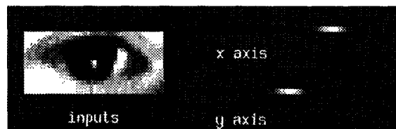
Figure 4: Image of the pupil and the eye socket, and the corresponding target outputs. 15 x 40 input image shown.
