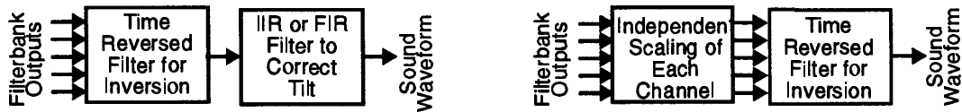
Figure 4. Two approaches are shown here to invert the filterbank. The left diagram shows the normal approach, the right figure shows a more efficient approach where the spectral-tilt filter is converted to a simple multiplication.
