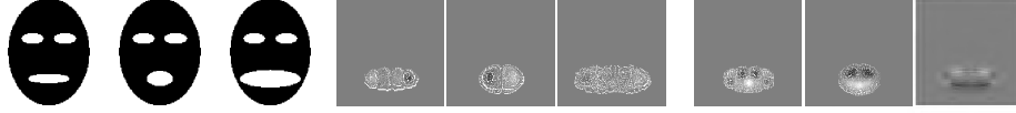
Figure 2: Synthetic image sequence examples (left). Mouth parameters are functionally related to one audio signal. Flow fields horizontal component (center) and vertical component (right).
