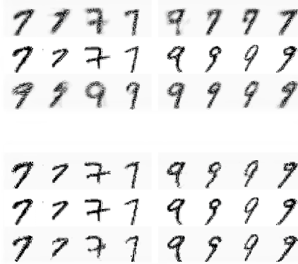
Figure 2: Cross reconstruction of 7s and 9s with models containing 25 hidden units (top) and 100 hidden units (bottom). The central horizontal line in each block contains originals, and the lines above and below are reconstructions by the 7s and 9s models respectively. Both models produce stereotyped digits in the small net and much better reconstructions in the large one for both the digit classes. The 9s model sometimes tries to close the loop in 7s, and the 7s model tries to open the loop in 9s.
