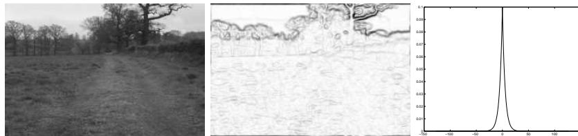
Figure 1: Distributions on images vs. distributions on features. Left and center panels show a natural image and its image gradient magnitude map, respectively. Right panel shows the empirical histogram (i.e. a distribution on a feature) of the image gradient across a dataset of natural images. This feature distribution can be used to create a MRF distribution over images[10]. This paper introduces the g -factor to examine connections between the distribution over images and the distribution over features.
