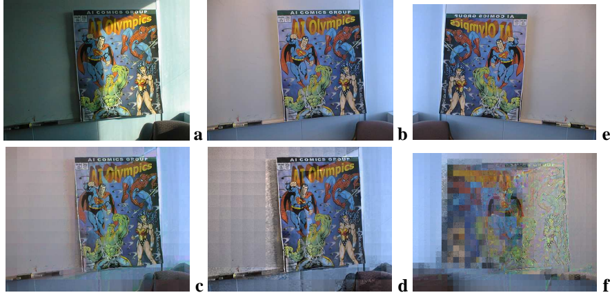
Figure 5: Modeling lighting changes with color flows. a. Image with strong shadow. b. Same image under more uniform lighting conditions. c. Flow from a to b using eigenflows. d. Flow from a to b using linear . Evaluating the capacity of the color flow model. e. Mirror image of b . f. Failure to flow b to e implies that the model is not overparameterized.
