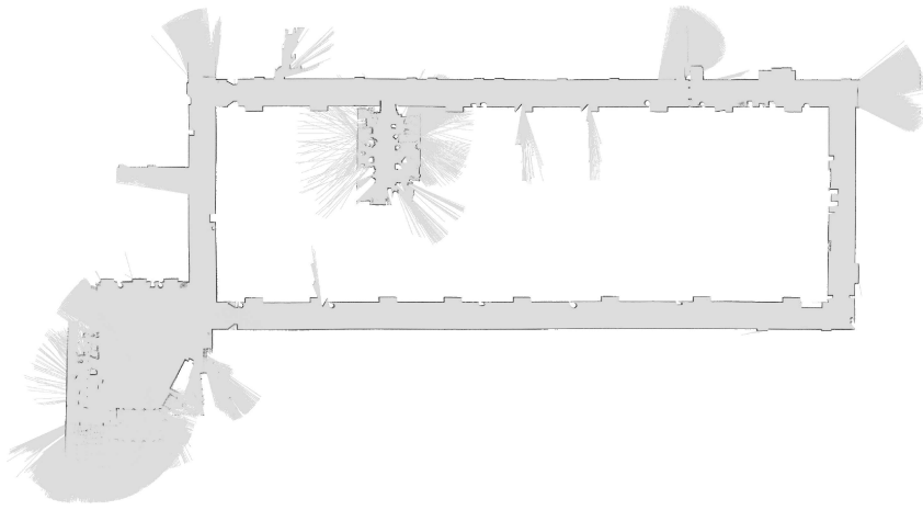
Figure 1: CMU's Wean Hall at 4cm resolution, using hierarchical SLAM. Please zoom in on the map using a software viewer to appreciate some of the fine detail.
