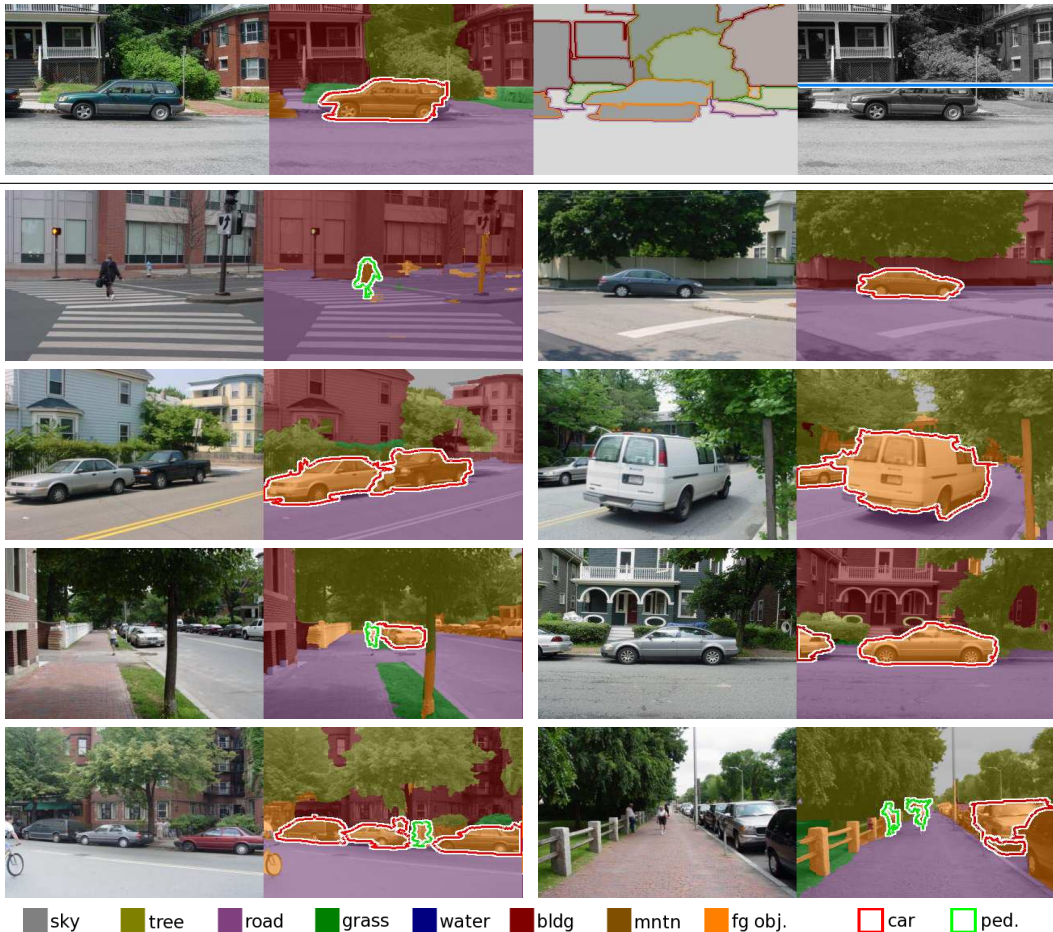
Figure 4: Qualitative results from our experiments. Top row shows original image, annotated regions and objects, region boundaries, and predicted horizon. Other examples show original image (left) and overlay colored by semantic class and detected objects (right).
